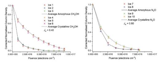
**Figure:** 2 keV electron-induced decay rates for the amorphous and crystalline solid phases of CH3OH (*left*) and N2O (*right*) astrophysical ice analogues at 20 K.
